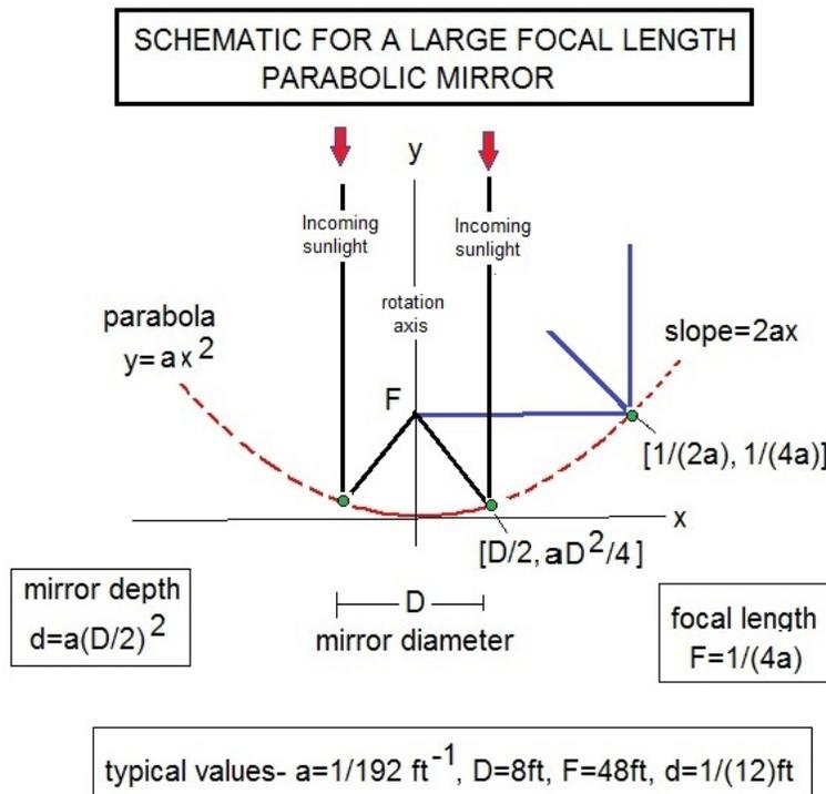
The mirror as shown is one of diameter  $D$  and focal length  $F$ . One can also consider  $D$  to be the side length when dealing with a square cross-section mirror. The axisymmetric parabolic surface can be defined as –
