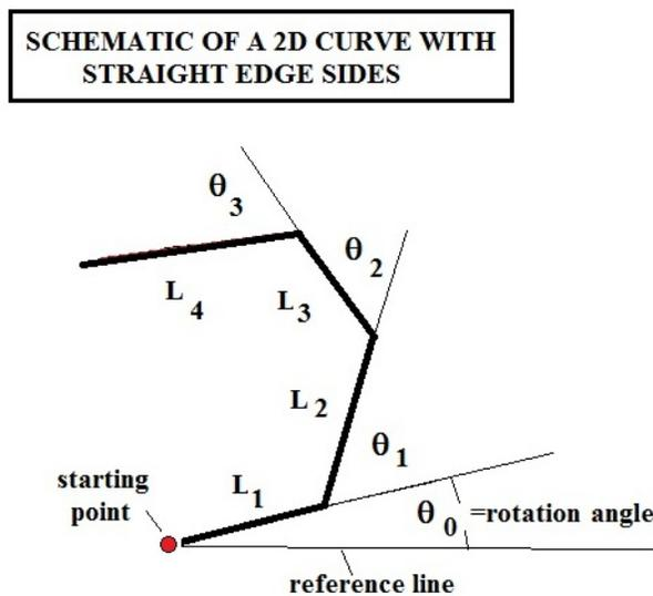
Once the angle of the first line is specified, all other lengths are uniquely defined by their length  $L_n$  and the angle  $\theta_n$  they make with respect to the next line segment  $L_{n+1}$ . For a curve which becomes closed after  $n$  elements have been connected, the sum of the angles of such polygons will always add up to  $2\pi$  radians. The concatenation of  $n$  lines each with its own specified angle forms the sequence-
