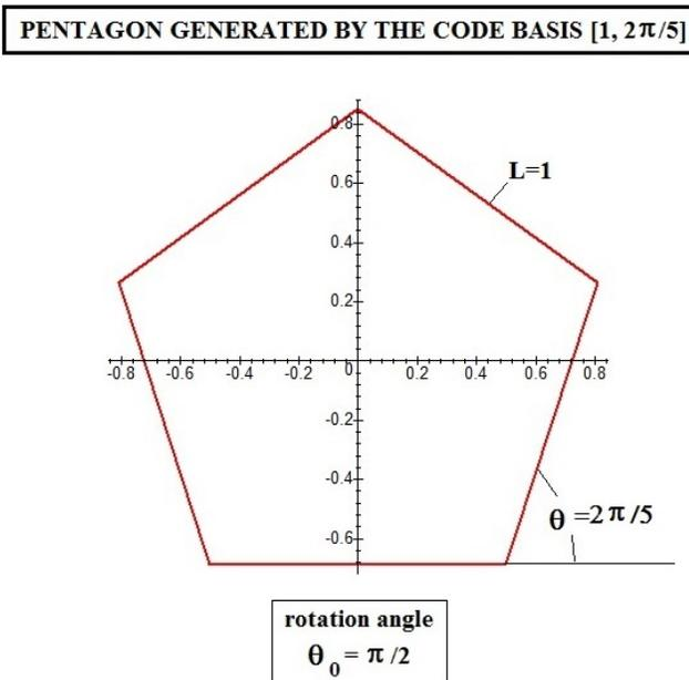
Notice we had to add a starting angle of  $\pi/2$  to get the bottom element to lie horizontal. The pentagon has an area of  $A=5/(4 \tan(\pi/5))=1.720477$ . To accomplish a magnification of this pentagon curve one simply needs to multiply  $L=1$  by  $k$ . A rotation of  $\varphi$  radians from the present orientation is gotten using a  $\theta_0 = \pi/2+\varphi$ . So a magnification by a factor of two and a  $\pi$  radian rotation produces the upside down pentagon-
