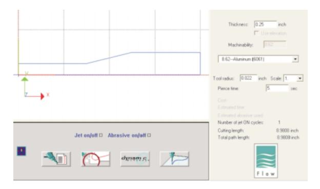
Figure A-14. Part loaded with no moves in Z-direction
