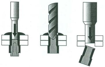
Figure 5a-3. Removal process for blind rivets
