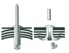
**Figure 5b-5.** The 'peeling' action of the shell provides a strong, reliable fix in softer materials.
