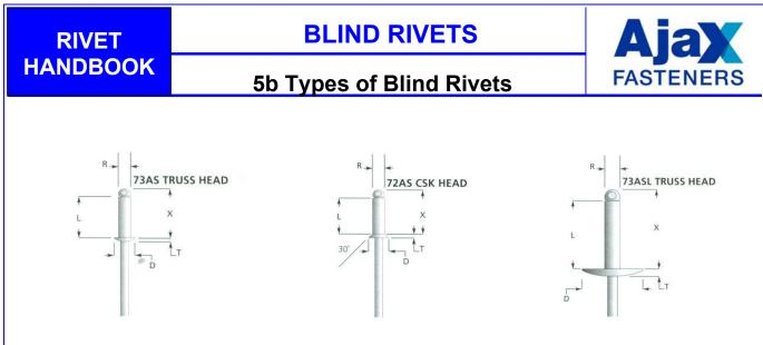
Figure 5b-2. Blind rivets have three basic head styles.
