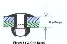
• If the grip range is too large (rivet is too short), insufficient material may be left on the blind side to secure the joint.
