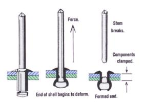
Figure 5a-1. The rivet is set by drawing the stem through the shell
