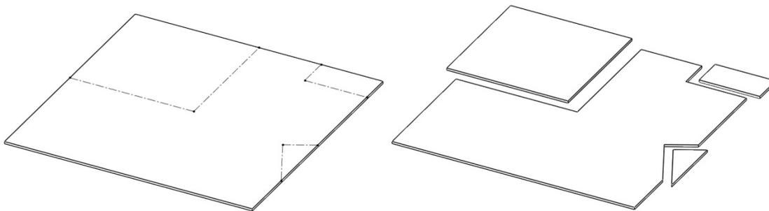
4. **DoALL bandsaw.** Creates cut from edge of part. The cut is not required to be straight, however, it cannot have a radius tighter than 4". If possible, use other sheetmetal cutting tools since this process is slow and has low precision. The width of the cut is ~1/16".
