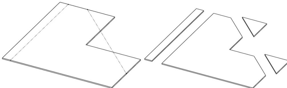
2. **Hand shear.** Partially shears a part.
