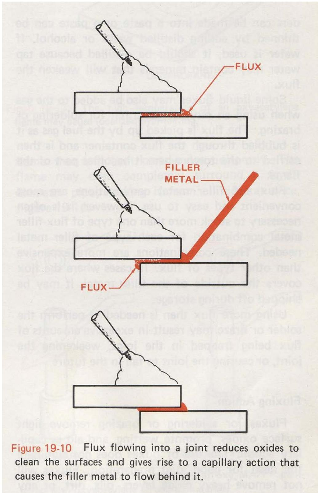
**Figure 19-10** Flux flowing into a joint reduces oxides to clean the surfaces and gives rise to a capillary action that causes the filler metal to flow behind it.
