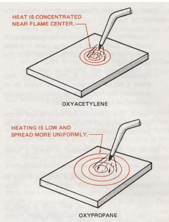
Figure 19-13 The high temperature of an oxyacetylene flame may cause localized overheating.
