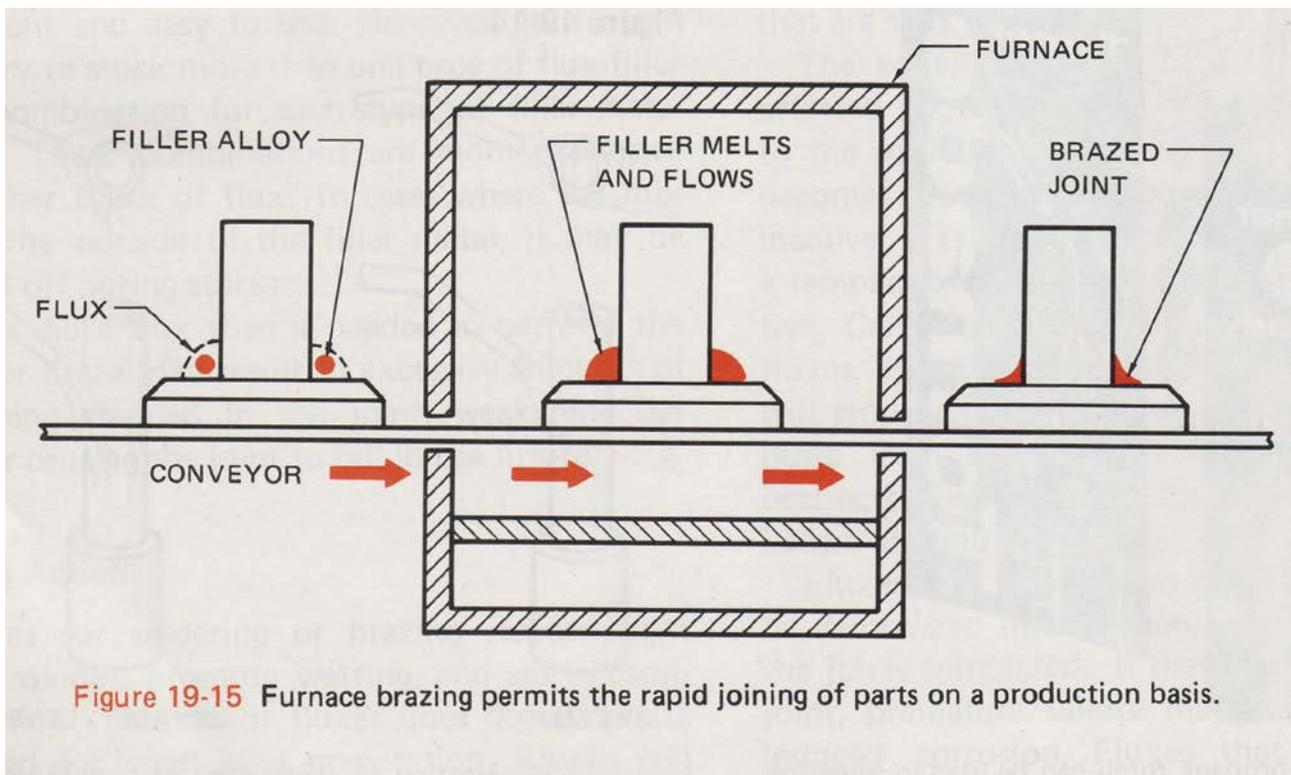
**Figure 19-15** Furnace brazing permits the rapid joining of parts on a production basis.
