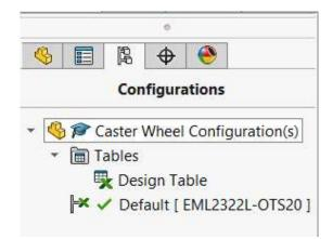
Fig. 3. ConfigurationManager tab showing all options for the caster wheel.
