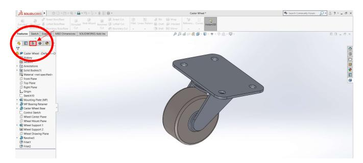
Fig. 2. Image of SolidWorks workspace, pointing to the ConfigurationManager tab.
