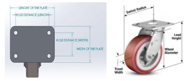
Fig. 1. Different views of a caster wheel with dimension annotations detailed above.
