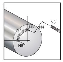
(Assume pilot hole is already drilled.) N1T303 (Small End Mill) N2M19 (Orient Spindle) N3G00 Z0.5 N4G00 X1. N5M133 P1500 N6G98 G1 F10. Z-.25 (Plunge into pre-drilled hole) N7G05 R90. F40.(Make slot) N8G01 F10. Z0.5 (Retract) N9M135 N10 G99 G28 U0 W0
