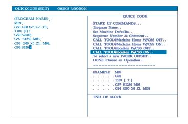
Programmed with the Start Up Command Selections Entered in with Quick Code for Tool 101.
