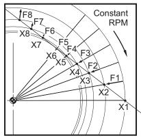
G32 motion includes both X feed rate and position commands at a constant RPM
