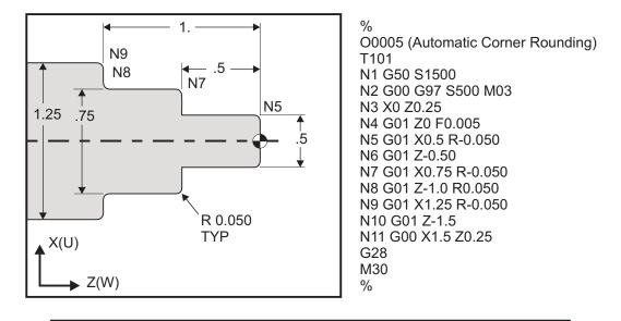
NOTES: 1) Incremental programming is possible if Ub or Wb is specified in place of Xb or Zb, respectively. So its actions will be as follows: X(POS<sub>current</sub> + i) = Ui, Z(POS<sub>current</sub>+k) = Wk, X(POS<sub>current</sub>+r)=Ur, Z(POScurrent+r)=Wr.
