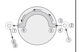
Example #1 M154 G00 G98 (feed/min) X2.0 Z0 C90 G01 Z-0.1 F6.0 X1.0 C180. F10.0 X2.0 G00 Z0.5 M155
