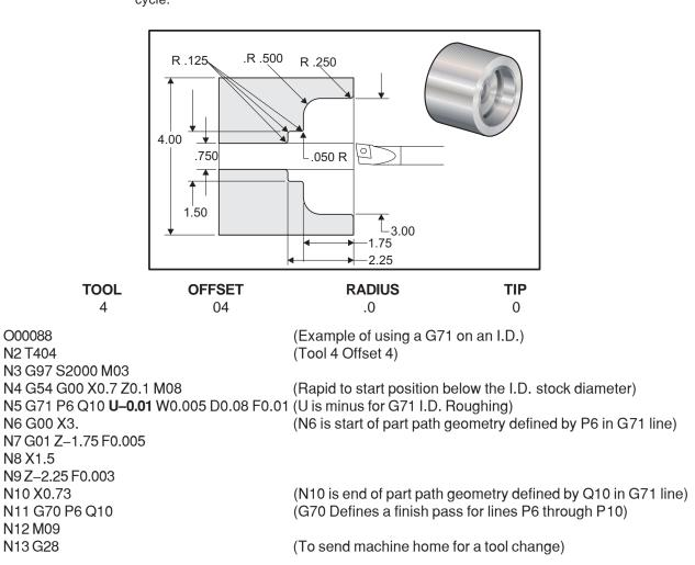
**NOTE:** Be sure the start position of the tool is positioned below the diameter of the part you wish to start roughing out, before defining a G71 on an I.D. with this cycle.
