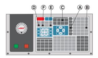
6. Press Ofset **(C)**, the Tool Geometry page should be displayed. If not page up until the Tool geometry page is displayed.
