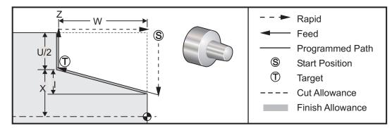
G90 is used for simple turning, however, multiple passes are possible by specifiing the X locations of additional passes.
