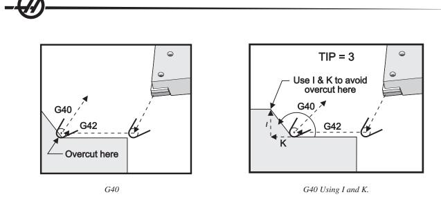
When address codes I and K are used in a G40 departure block, the control will use these values as an intersection for the end point of the last compensated cut. The following figure illustrates where I and K lie in relation to the departure stroke. Usually I and K lie along a face of the machined part.
