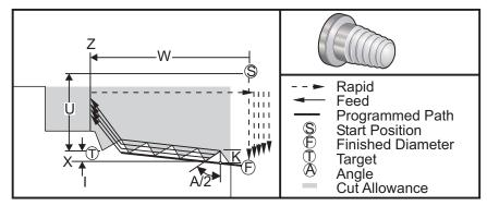
The G76 canned cycle can be used for threading both straight or tapered (pipe) threads.
