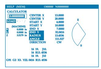
For inputs that have more than one solution, entering the last data value a second time will cause the next possible solution to be displayed. To change the CW value to the CCW value, highlight the CW/CCW column and press the Write/Enter button.
