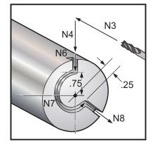
N1 T303 (Small End Mill) N2M19 N3G00 Z-.25 N4G00 X2.5 (Approach 2" diam stock) N5M133 P1500 N6G98 G01 X1.5 F40. (Cut to top of cam) N7G05 R215. X.5 F40. (Cut cam) N8G01 X2.5 F40. (Cut out of cam) N9M135 N10G99 G28 U0 W0
