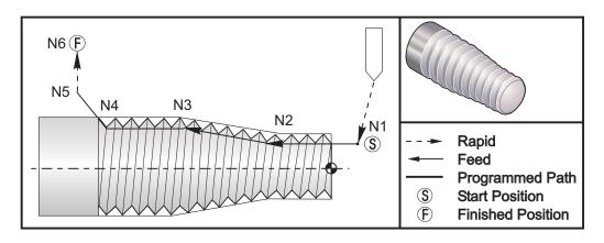
Straight-to-Taper-to-Straight Thread Cutting Cycle
