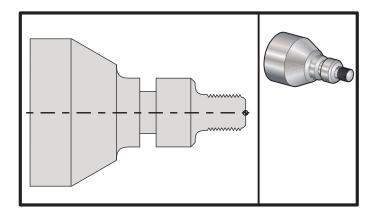
G76 Thread Cutting Cycle, Multiple Pass
