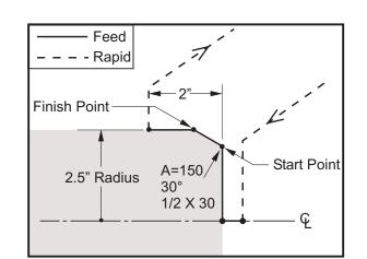
T606 G54; M03 S1500 G97; G00 X5. Z0.1; X0; G01 Z0 F0.01 G01 X4. Z0 F0.012;(start point) X5. (finish point) A150. (angle to finish point); Z-2.; X6.; G28; M30;
