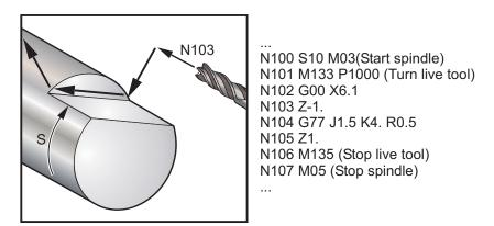
Cut a hexagon into the top half inch of a part that is three inches in diameter, using a tool half an inch in diameter:
