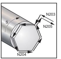
... N200 S10 M03(Start spindle) N201 M133 P1000 (Turn live tool) N202 G00 X4.5 N203 Z-0.05 N204 G77 J1.299 L6 R.25 N205 Z1. N206 M135 (Stop live tool) N207 M05 (Stop spindle)
