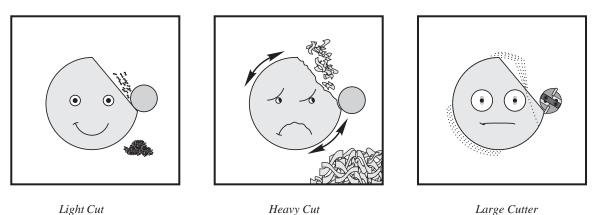
Heavy Cut The type of cut and the cutter will have an impact on part finish.
