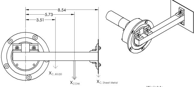
$\begin{aligned} &\text{Xcom} = ((X_{\text{C},80/20}) \times (W_{80/20}) + (X_{\text{C},\text{Sheet Metal}}) \times (W_{\text{Sheet Metal}})) / (W_{\text{Total}}) \\ &= (3.51 \text{in} \times 0.43 \text{ lbs} + 8.54 \text{ in} \times 0.34 \text{ lbs}) / 0.77 \text{ lbs} \\ &= 5.73 \text{ in} \end{aligned}$
