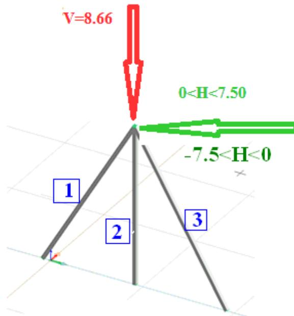
Figure 3: Three-bar truss problem in the case of two point loads at the top
