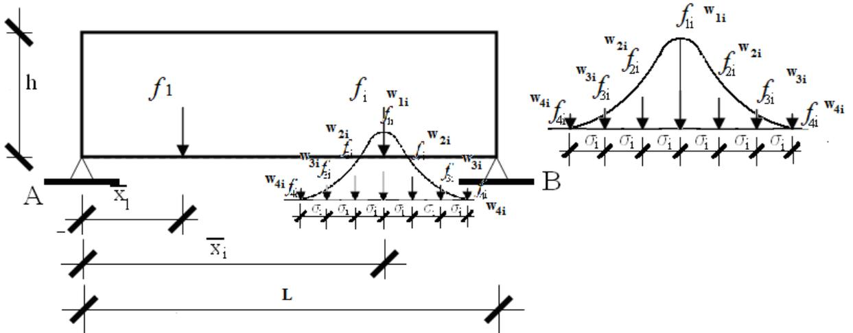
Figure 5: The design domain with the modified loadings and the corresponding probabilities
