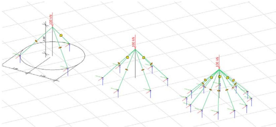
Figure 1: Alternative truss layouts in the case of a vertical point load at the top
