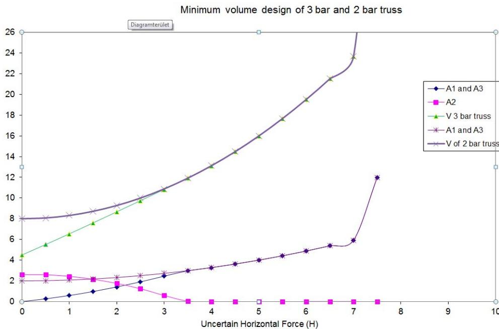
Figure 4: Optimal cross-sectional areas and minimum volumes of three and two bar truss problems
