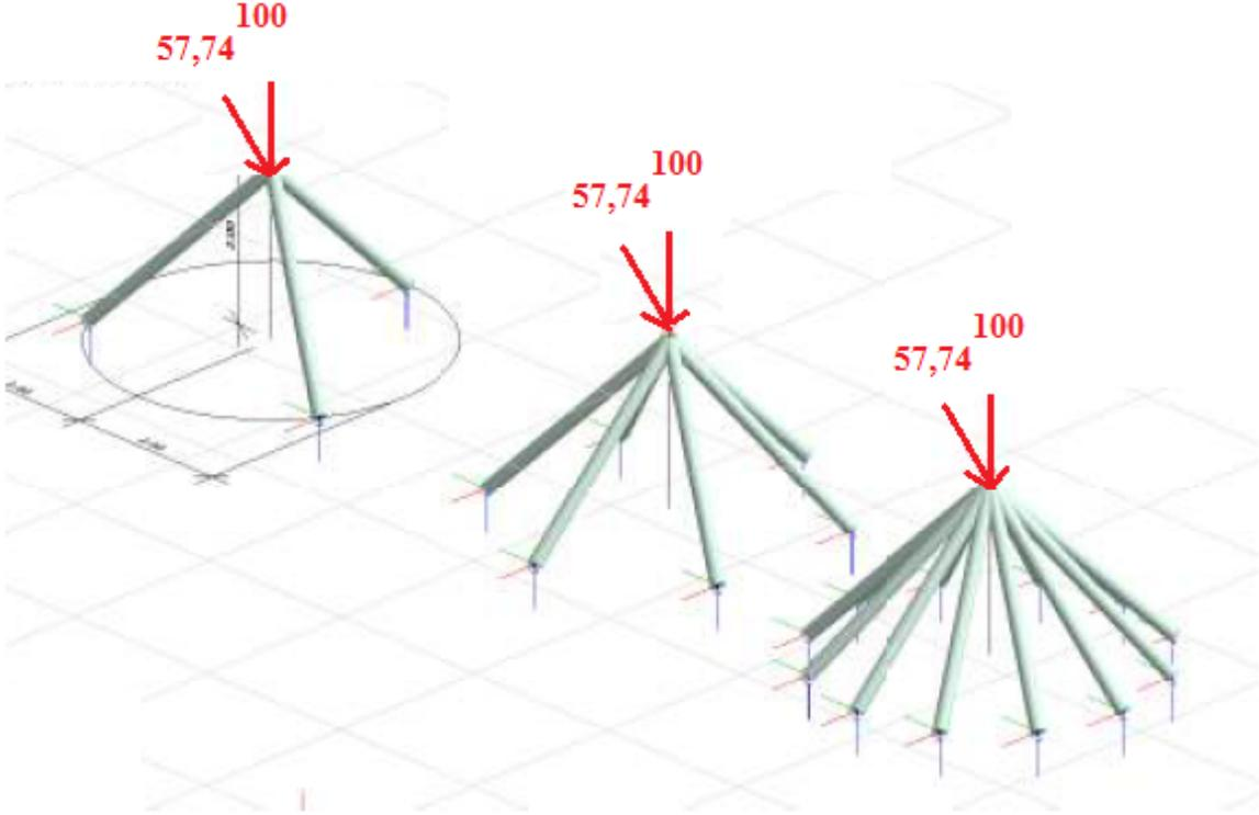
Figure 2: Alternative truss problems in the case of two point loads at the top
