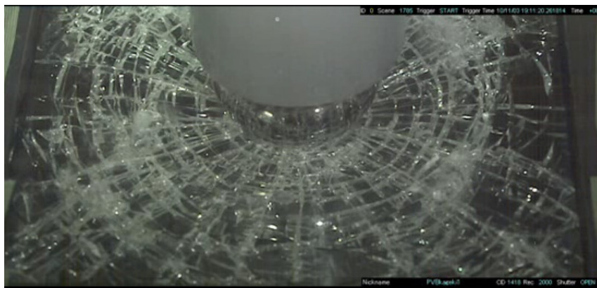
Figure 7: Dynamic fracture state of laminated glass by a high speed camera at 10ms
