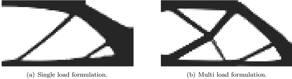
Figure 2: Cantilever beam optimum design obtained with the sensitivity filter in (a) single load and (b) multiple load formulations.
