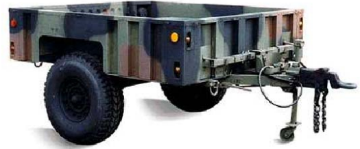
( a ) Army Trailer and Drawbar Assembly
