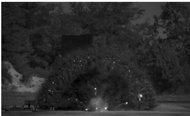
Fig. 1 Explosive dispersal of a solid particle bed using composition B as an explosive and steel particles
