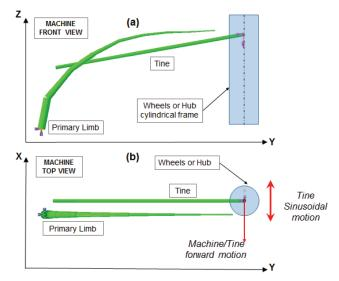
Figure 8. Interaction between a tine and a primary limb: (a) how the tine interacts with a primary limb and (b) the direction of forward and sinusoidal motion of the tine.
