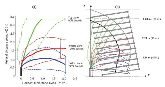
Figure 15. (a) Spatial distribution of limb prototypes of a hypothetical tree and (b) interaction of a canopy shaker with the limb prototypes.
