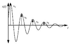
Figure 5. Underdamped response of a system having a SDOF.
