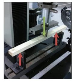
Figure 4. Three-point bending test of a citrus wood specimen (photo courtesy of Gupta).
