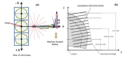
Figure 7. (a) Interaction of machine with a row of citrus trees and (b) set of tines in Y-Z plane interacting with primary limbs of citrus canopy.
