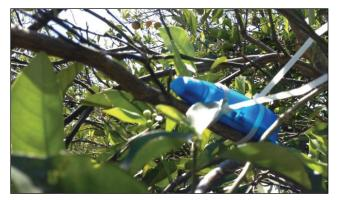
Figure 6. Accelerometer mounted on primary limb of a citrus tree.
