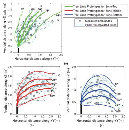
Figure 14. (a) Spatial modeling of limb prototypes for the (a) top zone, (b) middle zone, and (c) bottom zone.
