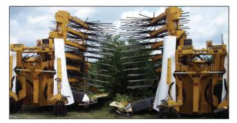
Figure 2. Continuous canopy shake and catch harvester (photo courtesy of Ehsani and Sajith).
