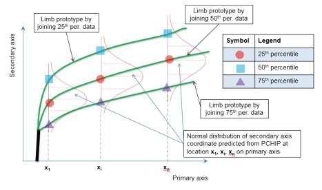
Figure 9. Method used to construct statistical limb prototypes from measured limb data.
