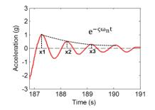
Figure 12. Underdamped response of a citrus tree limb.
