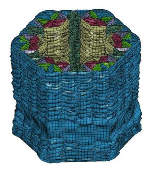
Fig. 12. Deformation mode of optimum with mass constraint 50% for Sections 5 under compression load.
