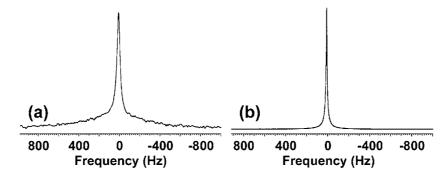
**Figure 6.** (a)  $^{25}$ Mg NMR spectrum of 2 mM Mg $^{2+}$  in 10 mg ml $^{-1}$  F-actin solution. The F-actin is uncondensed. (b)  $^{25}$ Mg NMR spectrum of 30 mM Mg $^{2+}$  in condensed 10 mg ml $^{-1}$  F-actin solution. F-actin is condensed into a bundled phase by the Mg $^{2+}$  ions. The solution Mg signal is large compared to the solid-state Mg signal.
