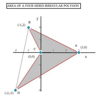
There are two ways to evaluate the area of this polygon. One can add together the areas defined by the sub-triangles ABC and DAC or one can subtract area DCB outside the polygon from the large triangle DAB. Using the second approach we find-
