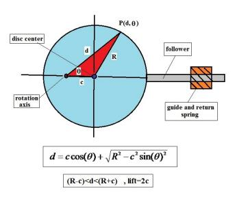
The disc rotates at constant angular velocity about a rotation axis which is locatred at distance c from the disc center. Applying the Law of Cosines one finds that-
