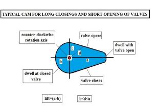
We can construct the follower response for this cross–section cam by measuring the distance d from the rotation axis of the cam surface at various angles. The measured displacement pattern over three 360 deg cycles looks like this-
