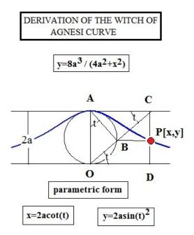
One starts with a circle of radius r=a and two horizontal parallel lines tangent to the top and bottom of the circle. Straight lines connect the points O, A, B, C, D and P as shown. The curve is defined such that point P(x,y) market as a red dot always lies on it. From the geometry one has at once that x=2a/tan(t), where the angle t is present in each of the three right triangles
